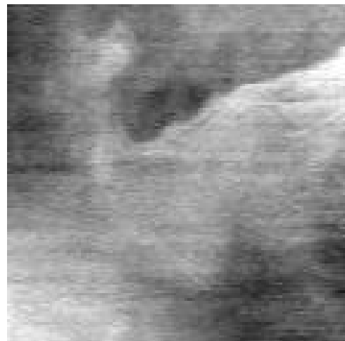
Figure 3-2: Sequence of in-phase SCA images around \nu = 4 . The scans are 3.3 \times 3.3 \mu m large. The smallest features displayed are consistent with the expected spatial resolution of the probe ( \approx 100nm ).
